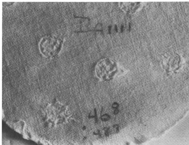
Figure 5. Fabric substrate after six applications of 0.1% slurry of moderately beaten wood pulp
